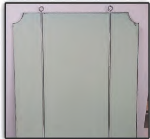
Welded Eye Bolts to Frame
